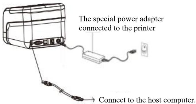
The special power adapter connected to the printer
